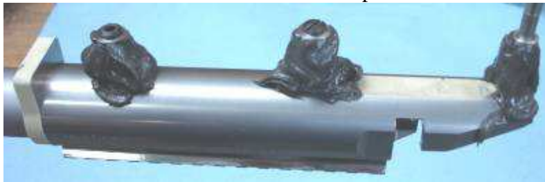
Picture # 7 mud on the pillars
