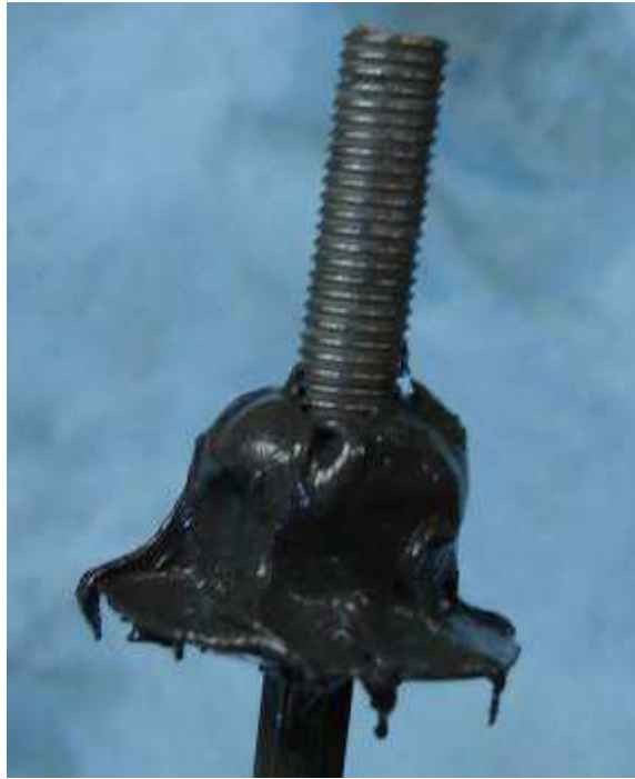
Showing the escutcheon & bolt with proper amount of mud. Bolt is sitting on an Allen wrench
