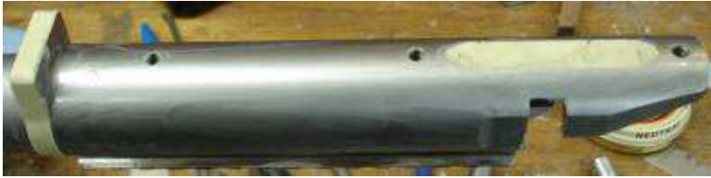
Putty & release agent before polishing, tape on lug
