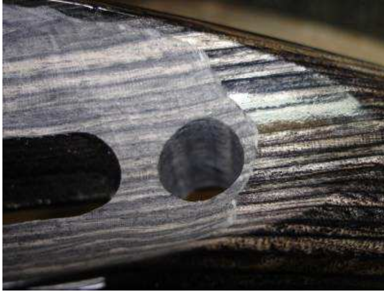
Pic # 4 Elevation wood left at tang. Be sure to leave some original wood for the action tang to sit on. (important)
